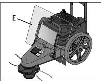
*Figure 3-1A: Debris shield in operating position.*
